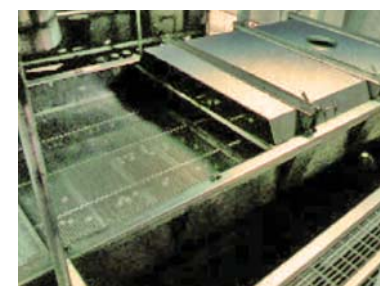
Easy Maintenance with Segmented Screen Decks and Top Cover
